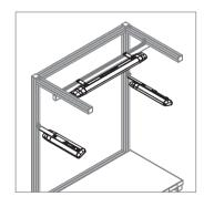
Rexroth's system lamp range provides glare and flicker-free light of the highest quality. For high-quality and even workstation lighting, the lamps can be operated individually or in combination with one another depending on the task. The lamps can be switched on and off when plugged into a socket with a power switch. Several lamps can be connected in series using the connection cables.
