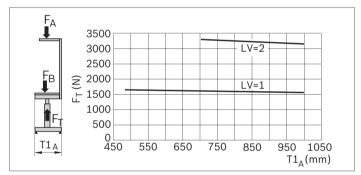
Bearing load for height-adjustable workstation where BA = 1000 mm. The bearing load decreases as the width BA increases. Standard load version LV = 1; heavy load version LV = 2; H3 = 0
