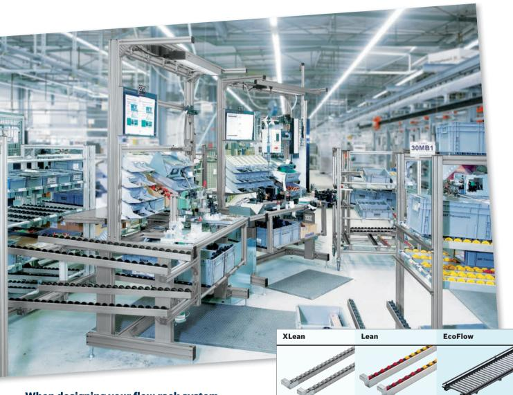
When designing your flow rack system, it is essential to know which materials will be supplied in what quantity and in which containers. The number of parts and containers, their type, their dimensions and their weight all need to be taken into account.
