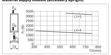
Bearing load for height adjustable material supply where BA = 1000 mm and H3 = 1200 mm. Standard load version LV = 4; heavy load version LV = 5
