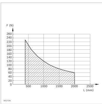
Diagram 1: Permissible load for the suspension profile
